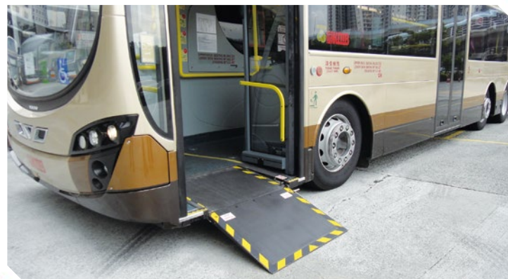
輪椅斜板 Wheelchair accessible ramp
