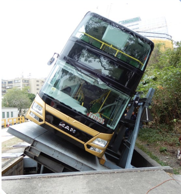
港珠澳巴士接受「傾斜」測試 A Hong Kong-Zuhai-Macao shuttle bus undergoing a tilt-test
