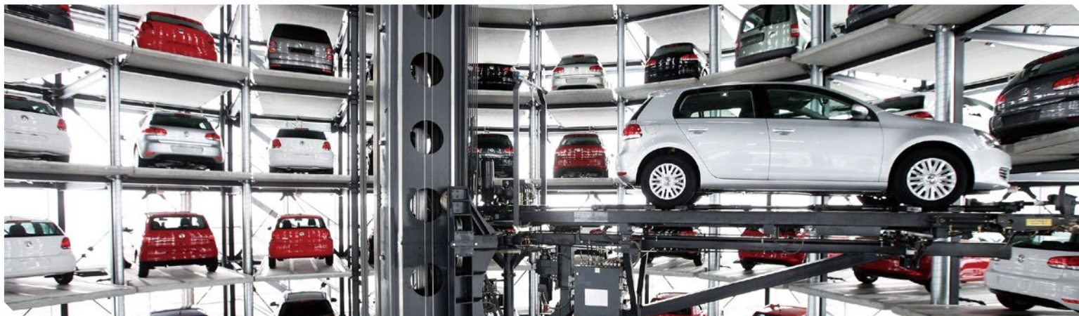
圓筒型 [原圖來源：Autostadt GmbH, Germany] Circular shaft lifting system [Source of the original photo: Autostadt GmbH, Germany]
