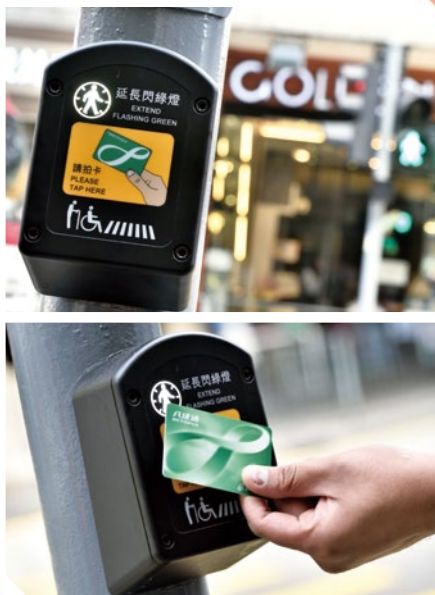
行人過路處供長者及殘疾人士試用的智能裝置 Smart devices at pedestrian crossings for trial by the elderly and people with disabilities
