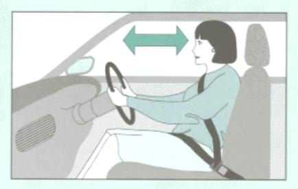
Do not place any objects over or near to the airbag outlet to avoid being hurt by these objects when the airbag inflates.
