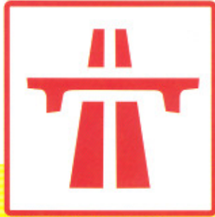
快速公路起點及其延續 Start and continuation of an expressway
