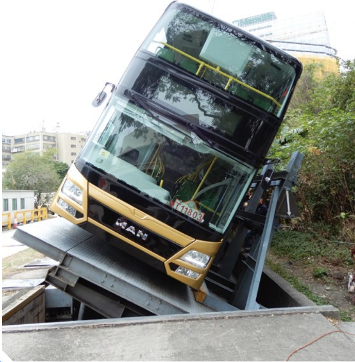
港珠澳巴士接受「傾斜」測試 A Hong Kong-Zuhai-Macao shuttle bus undergoing a tilt-test
