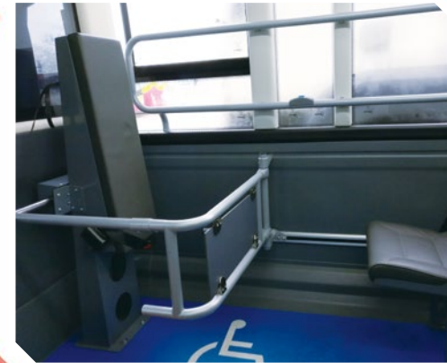
低地台輪椅小巴設有一個輪椅泊位 A low-floor wheelchair-accessible light bus with one wheelchair parking space
