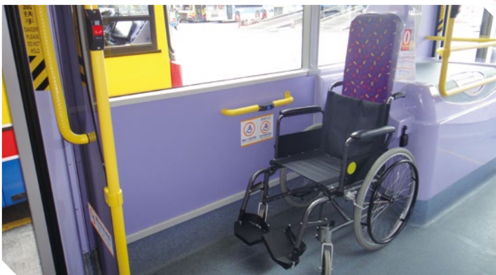
輪椅泊位 Wheelchair parking space
