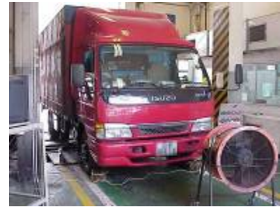
A Goods Vehicle Being Tested on a Dynamometer
