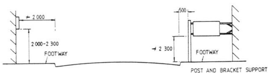
NOTES: (i) IF THE SPEED LIMIT IS GREATER THAN 50 km/h THE HORIZONTAL CLEARANCES WILL NEED TO BE INCREASED SEE PARAGRAPH 4.2.6.
