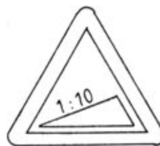
FIGURE No. 219 STEEP UPHILL GRADIENT AHEAD
