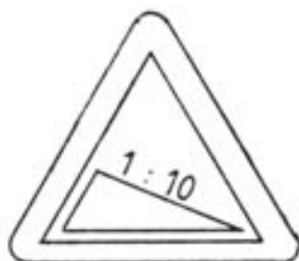
FIGURE No. 218 STEEP DOWNHILL GRADIENT AHEAD
