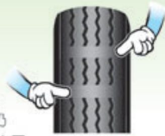
胎紋磨耗指示 Tread wear Indicator
