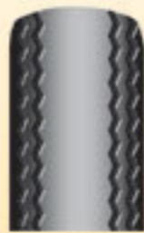
中間磨耗 Center wear
