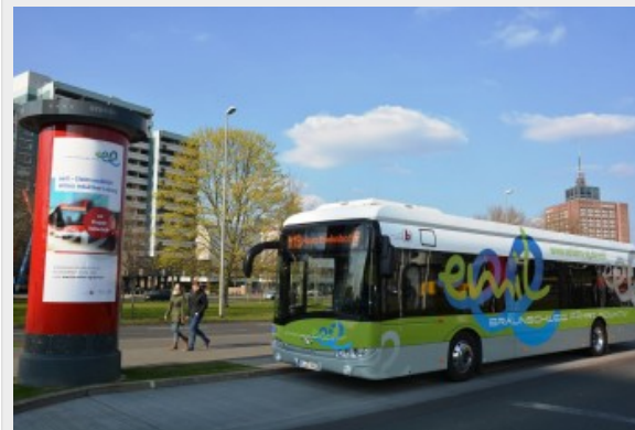
12m Solaris battery-electric bus with the PRIMOVE inductive charging system from Bombardier
