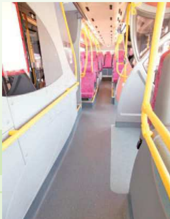
車廂地台使用防滑地台膠 Non-slip material is used in bus flooring
