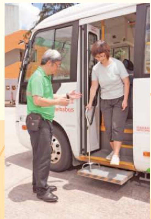
乘客可使用中門自動梯級上落 復康巴士 Passengers can get on and off rehabus by using auto- step at middle door
