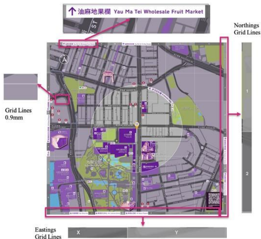
DIAGRAM 7.3.2.15 : LAYOUT OF GRID
