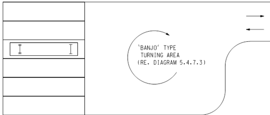
DIAGRAM 5.3.5.4: 45° PARKING SPACE - REVERSE INTO SPACE
