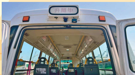
升降台操作指示灯 Warning signal during lift operation
