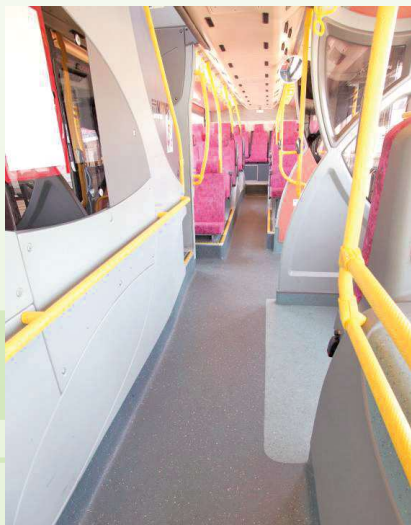
车厢地台使用防滑地台胶 Non-slip material is used in bus flooring
