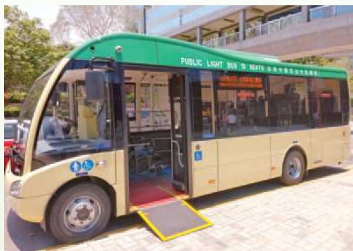
可供轮椅上落的低地台小巴 Low-floor wheelchair accessible Public Light Bus
