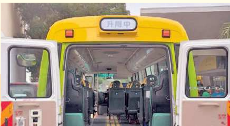
升降台操作指示燈 Warning signal during lift operation
