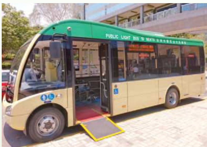
可供輪椅上落的低地台小巴 Low-floor wheelchair accessible Public Light Bus
