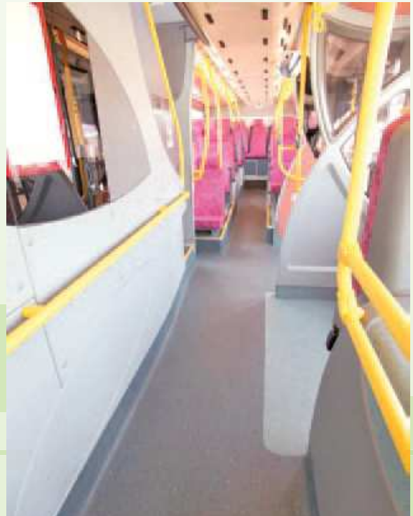
車廂地台使用防滑地台膠 Non-slip material is used in bus flooring
