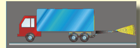
Sample layout of additional amber warning lamp (both rearwards and sideways or rearwards only: amber)
