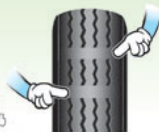
胎紋磨耗指示 Tread wear Indicator
